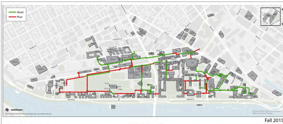
FIGURE 2: THE CAMPUS STEAM DISTRIBUTION NETWORK AND QUALITY. (SOURCE: MIT 2015 TOWN GOWN PRESENTATION TO THE CITY OF CAMBRIDGE)
